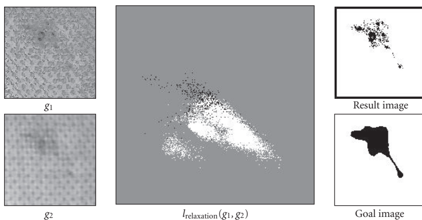
FIGURE 11.7. In the middle, the result of applying algorithm REL to two-operation images (left) and given goal image (bottom right) can be seen, and top right is the result of the application of this 2D-Lookup matrix to the two-operation images.
