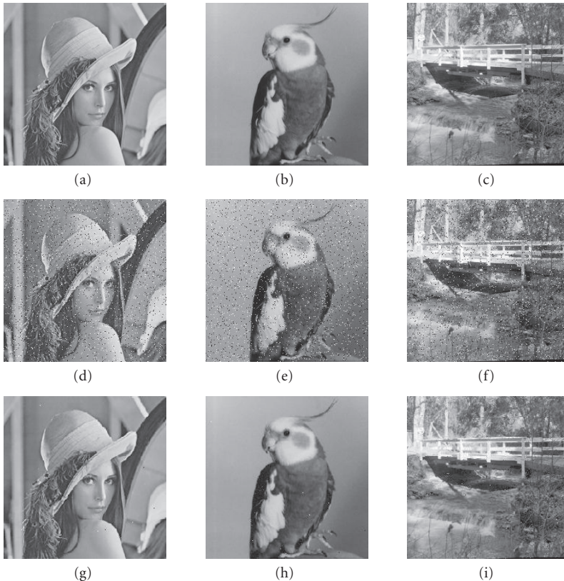
FIGURE 5.9. Original images (a), (b), (c), images with the salt and pepper noise from a test set (d), (e), (f), and images filtered using an evolved filter (g), (h), (i). The evolved filter was trained by means of Lena image (a), (d).
