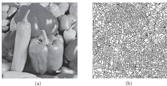
FIGURE 13.4. (a) Original peppers image ( 256 \times 256 ) and (b) its corresponding oversegmented watershed transformation.
